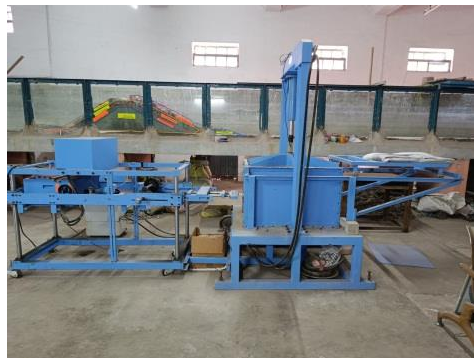
Geosynthetic pull out test equipment
