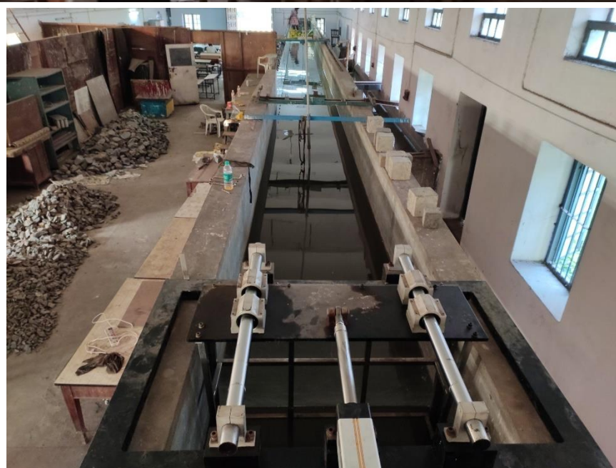
Wave flume with Wave Maker in Coastal Engineering laboratory
